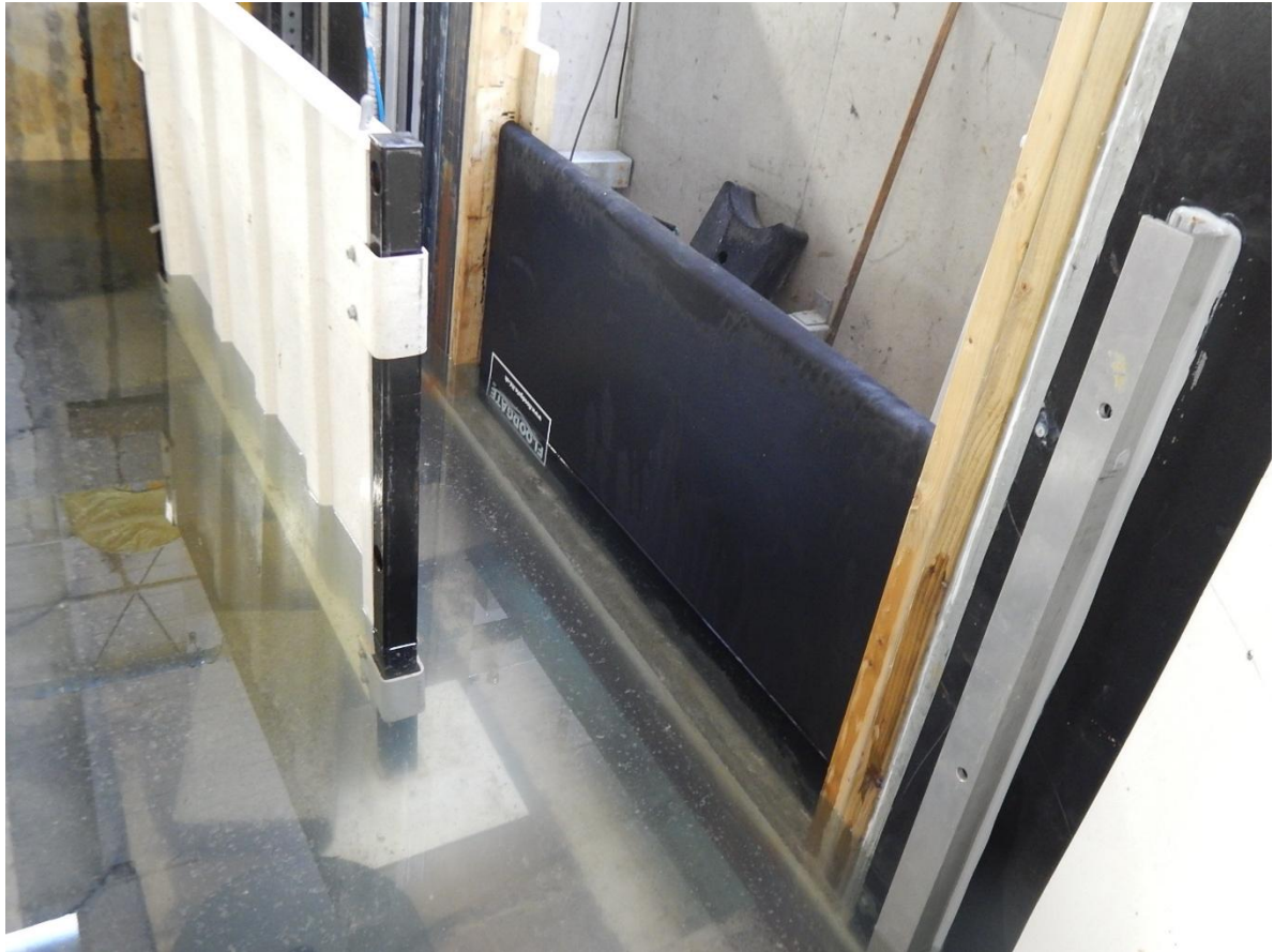
Figure 2 Static load test at 200 mm
