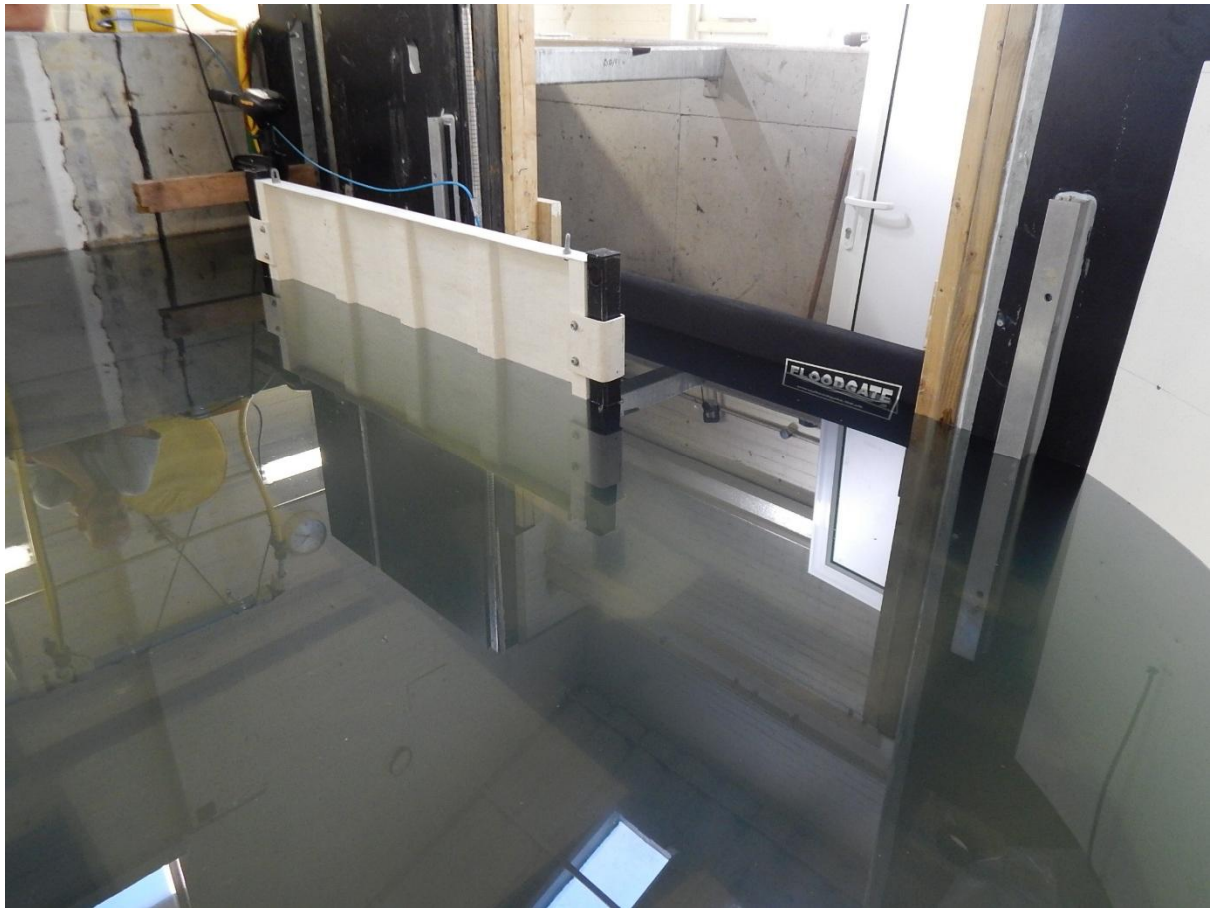
Figure 3 Static load test at 600 mm
