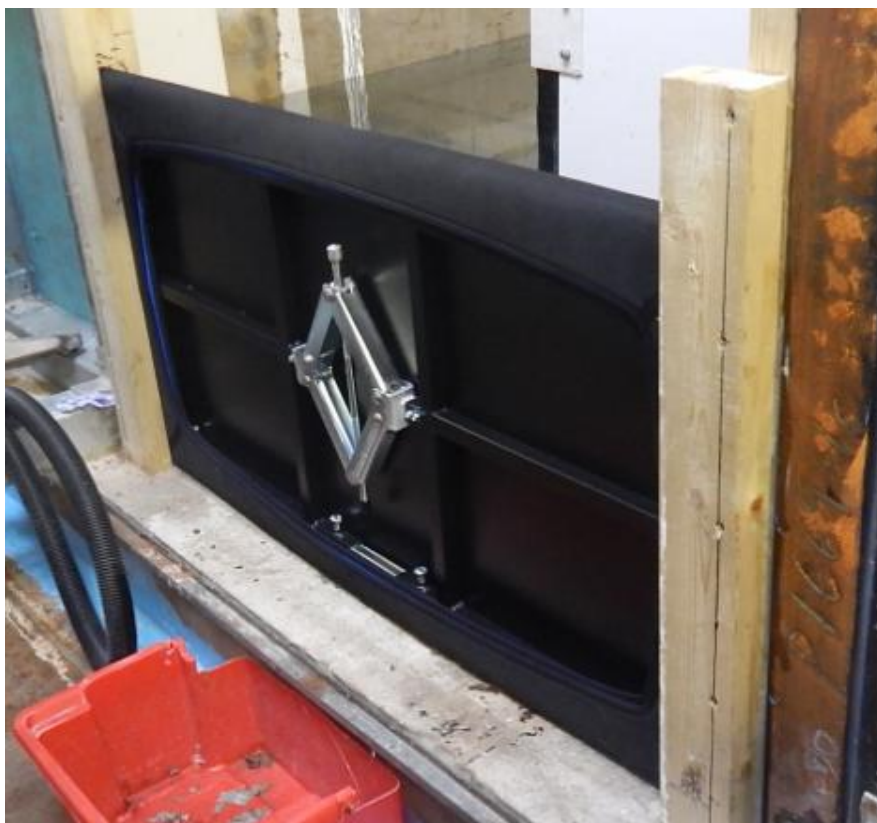
Figure 1 Floodgate product installed within flood tank (back face)
